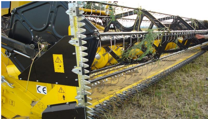
Picture 1. Active side dividers of the «rape tables» at combine New Holland CS-6090 at JSC "ANP Skopinskaya Niva"
