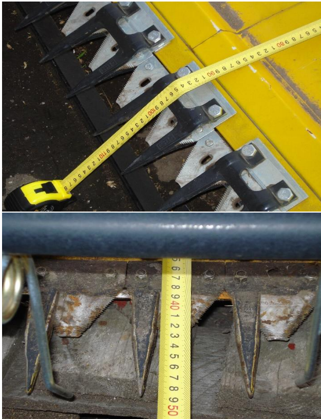
Picture 2. Depth of the device «rape table» (a) and reaper depth (b)
